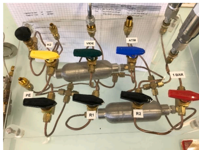
Fig. 6. Manual homemade Sieverts' apparatus developed at CNRS for in situ neutron diffraction studies. At the top: inlets for \text{H}_2(\text{D}_2) , vacuum ("Vide") and venting ("atm"). They are connected through copper capillaries and yellow, green and green valves, respectively, to the main body of the apparatus. Two pressure gauges (1 and 100 bar) are located at the top-right. The three black valves connect the sample colder (PE outlet) to two large reservoirs (R1 and R2).
