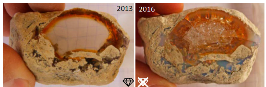
Figure 3. Example of an opal sample collected in 2013 at the mine site (Kok Woha, Wollo Province, Ethiopia, see [39] for details on mines) and the result after 3 years of storage in the atmosphere, where it was allowed to dry.
