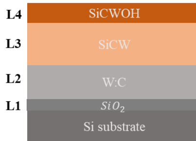
Figure 8: Sample layout considered for the interpretation of IBA simulations
