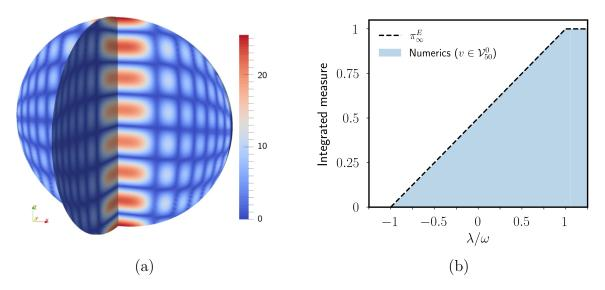
Figure 1: (a) Velocity magnitude ||v|| of an inertial mode with angular frequency  $\lambda \simeq 0.5412$  in the ellipsoid  $A_1 = A_2 = 1$  and  $A_3 \simeq 1.179$ , rotating at the angular velocity  $\vec{\Omega} = (0, 0, 1)$ . (b) Integrated probability measure of all the eigenvalues for  $v \in \mathcal{V}_{50}^0$  in the round ball [VSC20], which converges towards a uniform distribution.
