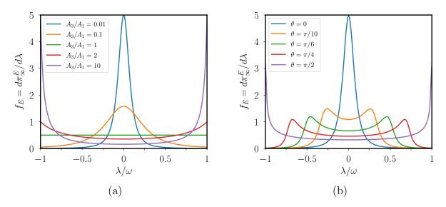
Figure 2: Non-vanishing density  $f_E$  for eigenvalues  $\lambda \in [-\omega, +\omega]$  obtained from theorem 7.1. (a) Formula (13) for integrable cases in axisymmetric ellipsoids with  $A_1 = A_2 = 1$  and  $\vec{\Omega} = (0, 0, 1)$ . (b) Numerical evaluation of formula (11 for non-integrable cases with a tilted vector  $\vec{\Omega} = (\sin \theta, 0, \cos \theta)$ in an axisymmetric ellipsoid  $A_1 = A_2 = 1$  and  $A_3 = 0.01$ .
