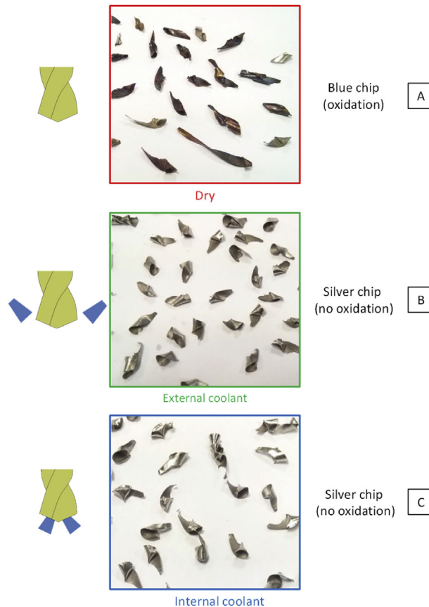
Fig. 4. Chips after drilling for the three lubrication conditions – A Dry conditions – B External coolant – C Internal coolant.
