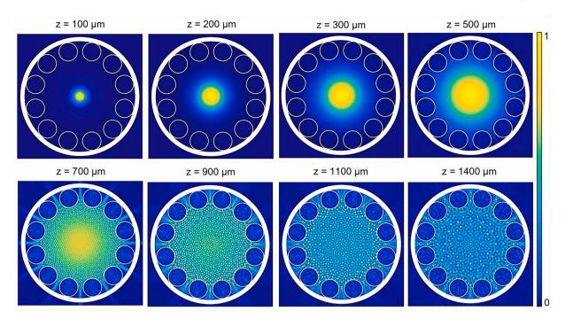
**Fig. 2.** Simulated evolution of the intensity distribution profile on the HCPCF cross-section along the z-axis at 543 nm. The color bar stands for the normalized intensity calculated for every image. Here, we define z = 0 as the position of the SMF extremity, as depicted in Fig. 1b.
