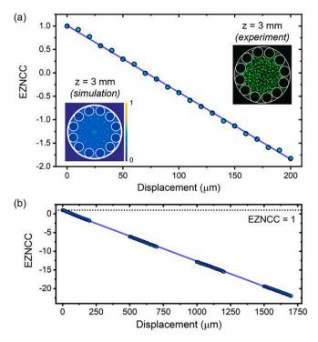
Fig. 6. Displacement sensing results. Plots of the EZNCC values as a function of the SMF displacement inside the HCPCF for a measurement range of (a) 200  $\mu$ m and for an extended range of (b) 1.7 mm. The extended range of 1.7 mm consists of several displacements between 500  $\mu$ m and 700  $\mu$ m, 1000  $\mu$ m and 1200  $\mu$ m, and 1500  $\mu$ m and 1700  $\mu$ m. Inset images stand for simulated and measured intensity distribution profiles at z = 3 mm.
