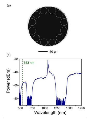
**Fig. 3.** (a) Cross-section of the 12-tube SR-TL HCPCF. (b) Transmission spectrum for a 4 m-long fiber. The vertical dashed line identifies the wavelength at which the experiments have been performed, 543 nm.
