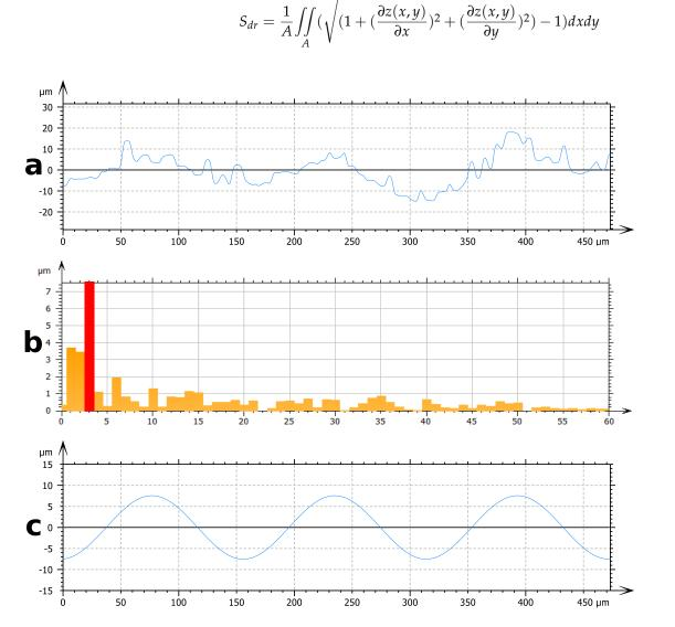
**Figure 3.** Example of frequency filtering by FFT: (**a**) unprocessed profile of Phyllostachys Bamboo leaf, (**b**) frequency spectrum with in red the selected frequency, and (**c**) filtered profile.
