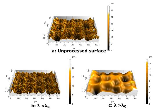
**Figure 4.** Example of Gaussian filtering, with a cut-off of 120 μm, on Phyllostachys bamboo leaf: (**a**) unprocessed surface, (**b**) filtered surface for small scales, and (**c**) filtered surface for high scales.
