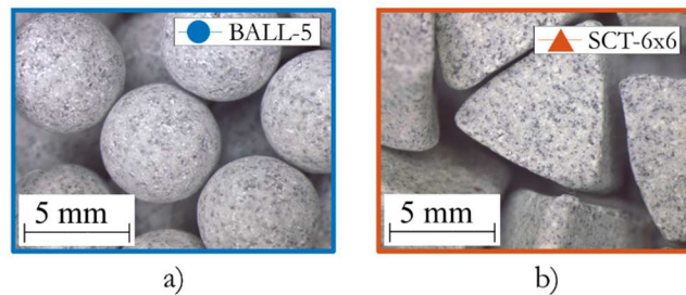
358 Figure 8. Ceramic abrasive media of different shape: a) spherical, \varnothing=5 mm, and b) pyramidal, dimensions=6x6 mm. Both medias had the 359 same composition and were provided by ABC SwissTech.
