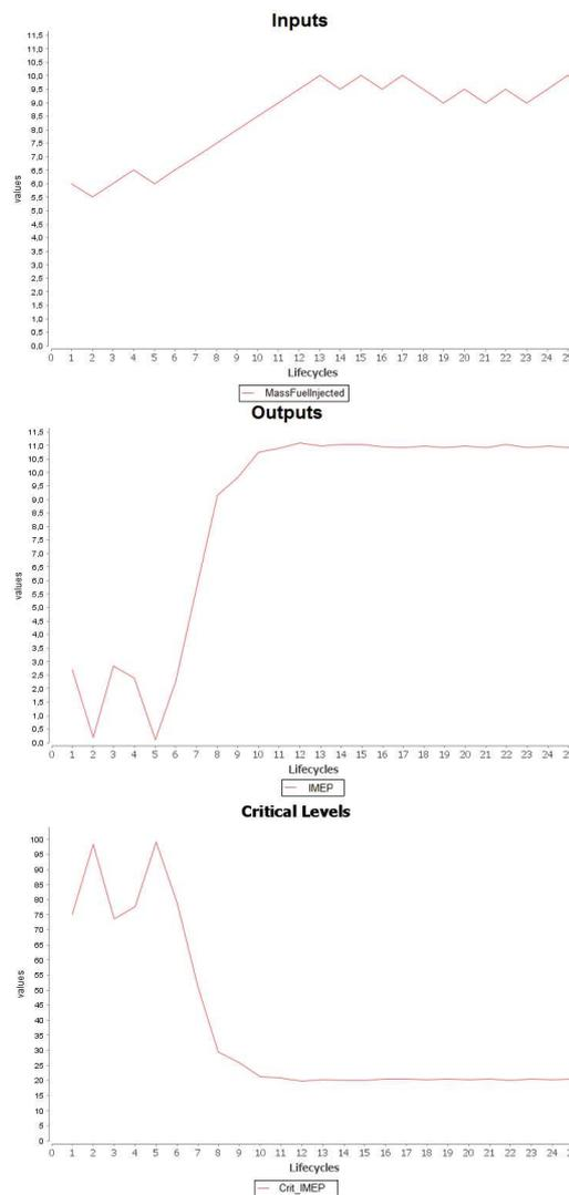
Figure 4: Controlling Injected Mass Fuel to Maximize IMEP
