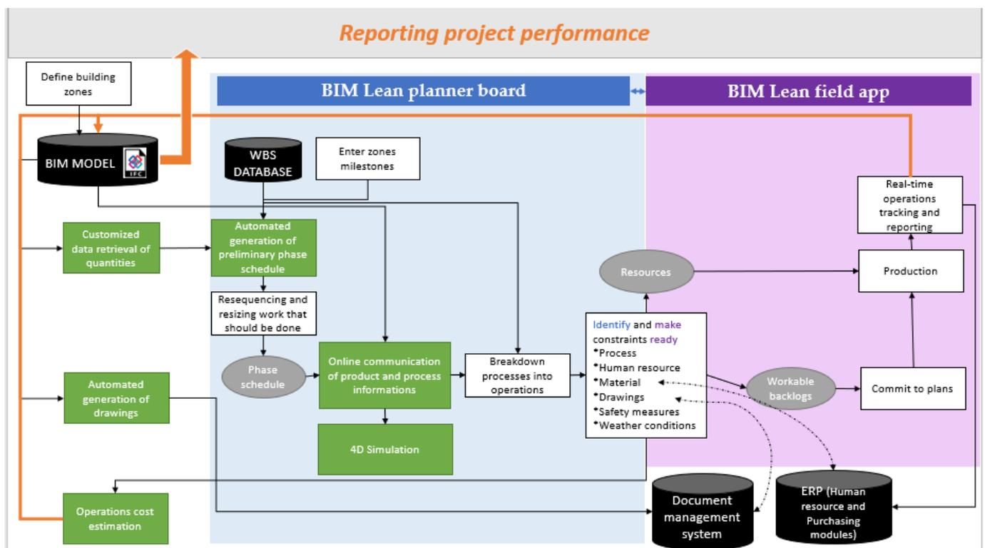
Figure 6. Detailed mapping of BIM functionality contributions along LPS process.
