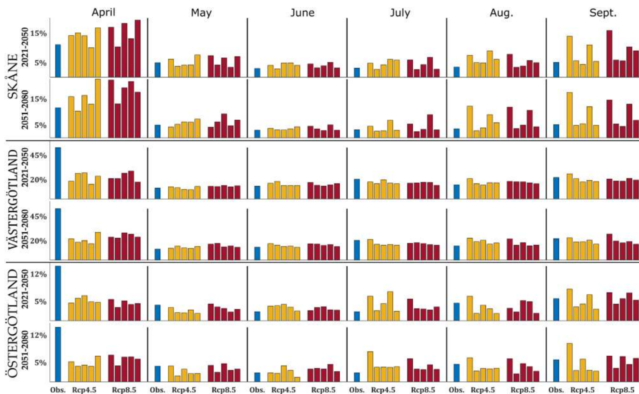
Fig. 9. Runoff as a percentage of total precipitation at the Skåne, Västergötland, and Östergötland sites. For each scenario, the five histograms represent the five different climate models as listed in Table 2. Note difference in vertical scale for Västergötland.
