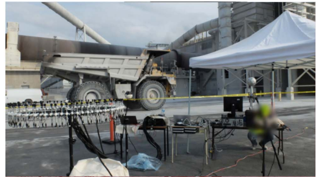
Figure 1. Sound environment capture in an open-air lime mine using a double-layer circular microphone array. Recordings were performed near a mine crusher (left) and with trucks passing at few meters from the array (right), among others.
