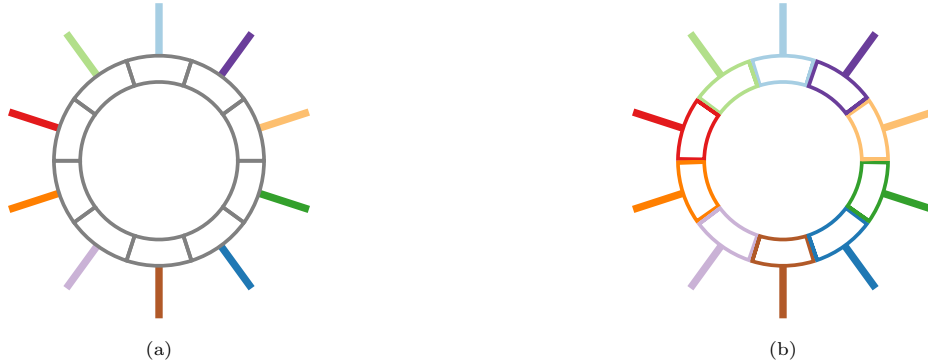
Figure 1: Two different patterns to introduce mistuning in bladed disc models where the different colors represent the deviations between sectors. In Fig. (a), the mistuning is applied on the blade and in Fig. (b) the mistuning is on all the sector.
