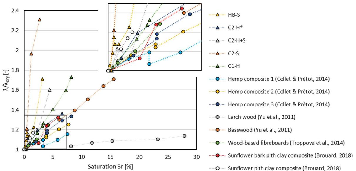
**Figure 10** Evolution of thermal conductivity (normalized to the dry thermal conductivity) with saturation rate of several materials from literature and from the present study.
