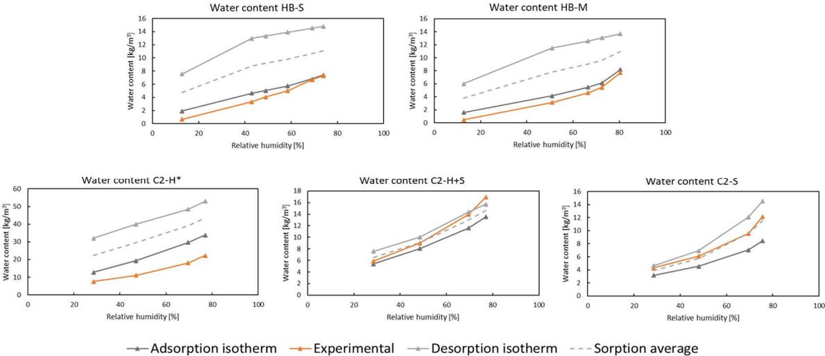
**Figure 14** Comparison between experimental water content and the water content corresponding to the relative humidity (calculated as the mean value of the relative humidity pair) for each permeability test according to the adsorption isotherm, the desorption isotherm, and the mean value of both.
