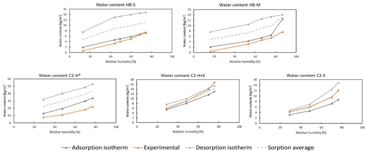
**Figure 15** Comparison between experimental water content and the water content corresponding to the relative humidity (calculated as the mean value between the upper and lower surface relative humidity) for each permeability test according to the adsorption isotherm, the desorption isotherm, and the mean value of both.
