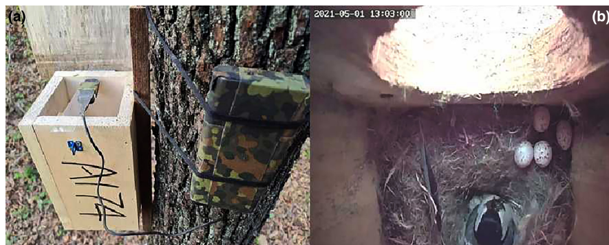
FIGURE 1 (a) Nest box monitoring setup showing a mini digital camera affixed under the roof of the box and connected with a cable to the external battery pack. (b) The Japanese tit returned to the nest to continue incubating after nest predation.
