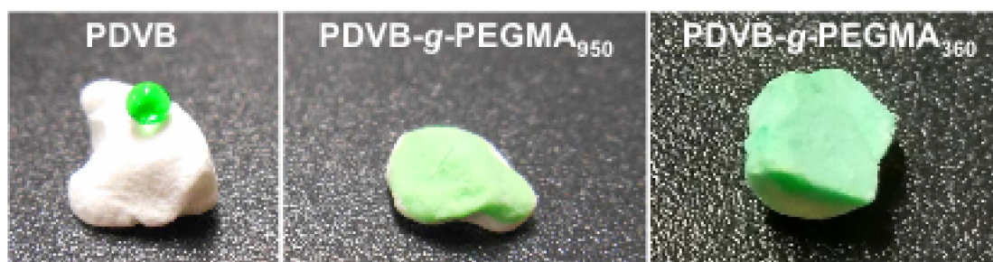
Fig. S2 An aqueous solution of green food dye spotted onto PDVB, PDVB-g-PEGMA 360 and PDVB-g-PEGMA 950 as an estimate of surface grafting
