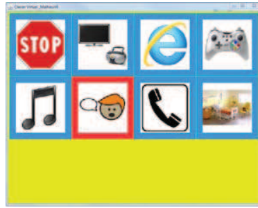
Figure 8. First layout of the Matthieu keyboard, column scanning
