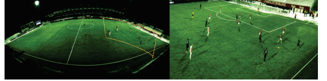
Figure 5: Panorama video with labeled ROI (left) and the virtual camera generated (right). It can be observed that it is not a simple crop from the bigger video.
