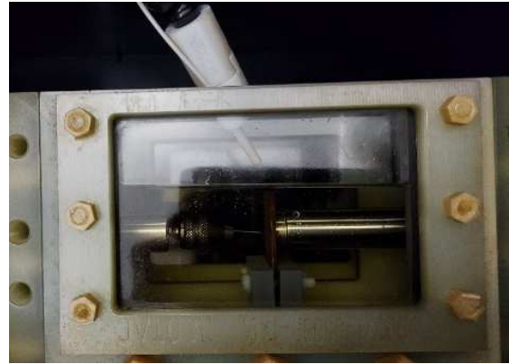
Fig. 1 Photograph of the DUT with needle-pressboard plane configuration filled with ester and the orientation of the EO probe used for PD tests
