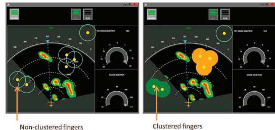
Figure 1- a) (left) 3 input device detected; b) (right) output of the clustering of two input devices (merged disks bottom left)
