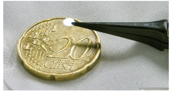
FIG. 13. A prototype 2-mg fused silica mirror with a diameter of 3 mm and a thickness of 0.1 mm. A high reflective coating with a thickness of around 6 \mu\text{m} and a transmission of 10 ppm is deposited.
