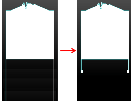
Fig. 13: Modification on the crevice region, before (left) and after (right).
