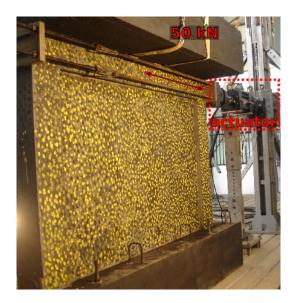
**Figure 3.** Masonry infilled frame before the experiment. The hydraulic actuator is shown in the dashed red box. The 50 kN dead load is visible above the frame.
