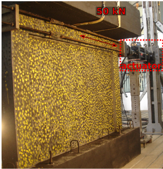
Figure 3. Masonry infilled frame before the experiment. The hydraulic actuator is shown in the dashed red box. The 50 kN dead load is visible above the frame.
