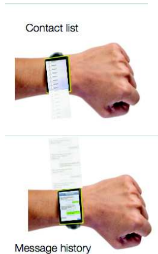
Figure 3. Combining both displays can extend the overall display space of the devices.
