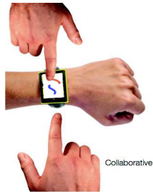
Figure 2. The HWD camera can sense the direction of finger landing on the smartwatch for multi-user sensing.
