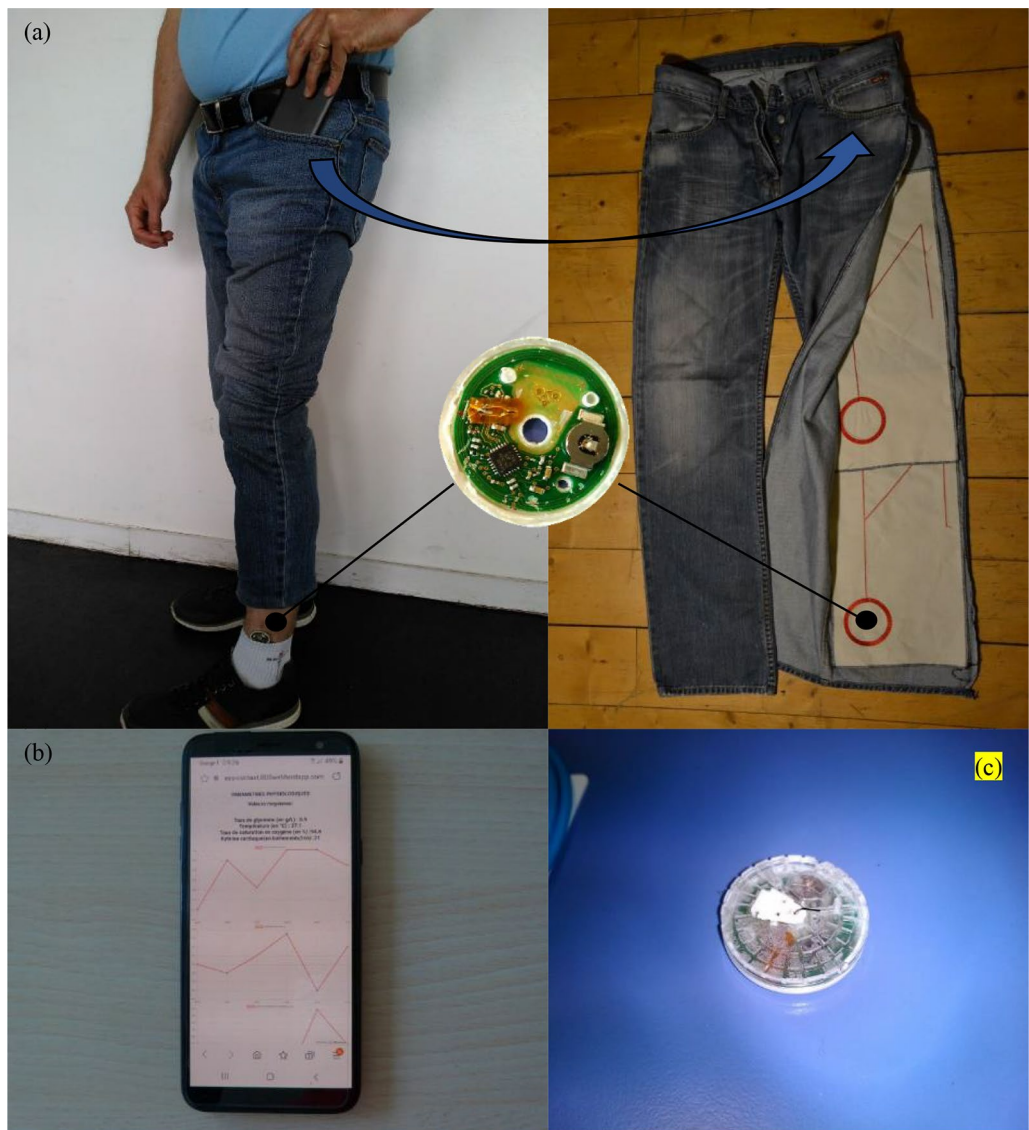
Figure 7. (a) The textile dual-band near field multiple combiner proof of concept, (b) the data transmitted and (c) the sensor.
