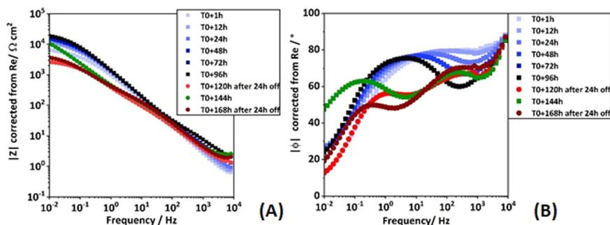
**Fig. 12 Bode diagrams obtained regularly during the 7 days of cathodic polarization with two interrupted phases (the 5th and 7th days).** The modulus in (A) and phase in (B) are plotted in function of the frequency and corrected from the “Re” (Electrolyte Résistance), for unpainted DH36 steel immersed in naturally aerated artificial seawater and in static conditions at 20 °C.
