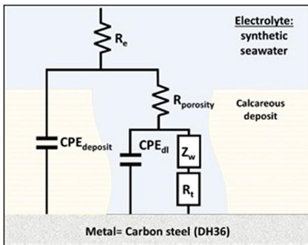
**Fig. 9** The EEC model represents the interface of unpainted DH36 steel/seawater under continuous or interrupted cathodic protection. This EEC model is valid at room temperature, under static conditions, and with artificial naturally aerated seawater.
