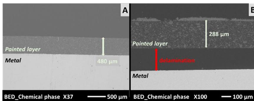
**Fig. 5 Scanning Electron Microscope (SEM) pictures of different samples cross-sections at different stages of paint degradation.** In (A), the case of freshly painted DH36 steel without defects and, in (B), a painted DH36 steel aged after 597 days of immersion. Both are immersed in artificial seawater at 20 °C naturally aerated in static condition. These images are obtained by Energy Dispersive X-ray Spectroscopy (EDS) using a Backscattered Electron Detector (BED).
