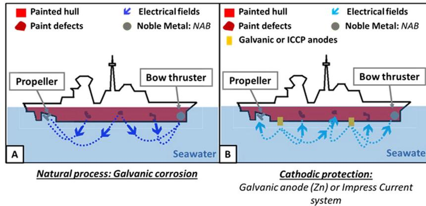
**Fig. 1** Illustration of the major causes of electrical signature of ship's hull. There are two cases, the natural and spontaneous phenomenon, the galvanic coupling illustrated in (A), and the process of cathodic protection illustrated in (B) with the case of Impress Current Cathodic Protection system (ICCP)<sup>4</sup>.
