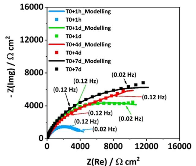
**Fig. 10** Nyquist diagrams measured during 7 days of cathodic polarization at  $-0.8$  V versus SCE. Imaginary ( $Z(\text{img})$ ) is plotted in function of the real parts ( $Z(\text{Re})$ ) of the impedance, under static, at  $20$  °C in natural aeration and static conditions, after 1 h, 1 day, 4 days and 7 days of continuous cathodic polarization.
