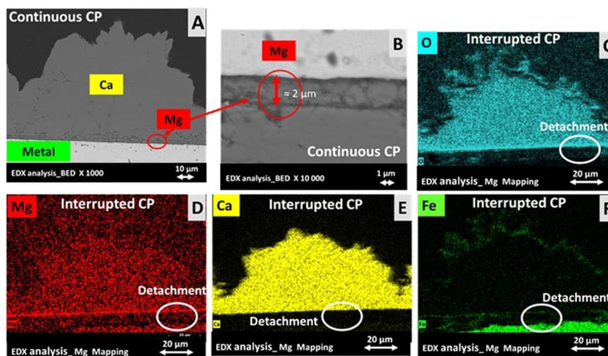
**Fig. 6 SEM pictures of the seawater/metal interface state during continuous or interrupted cathodic protection.** In (A, B), cross-sections of the sample obtain after continuous cathodic protection for 7 days in natural aeration, at 20 °C in static conditions. In (C–F), cross-sections pictures of a sample obtain after two interruptions of the cathodic protection, in natural aeration, at 20 °C, under static conditions. EDX mapping of the elements is performed.
