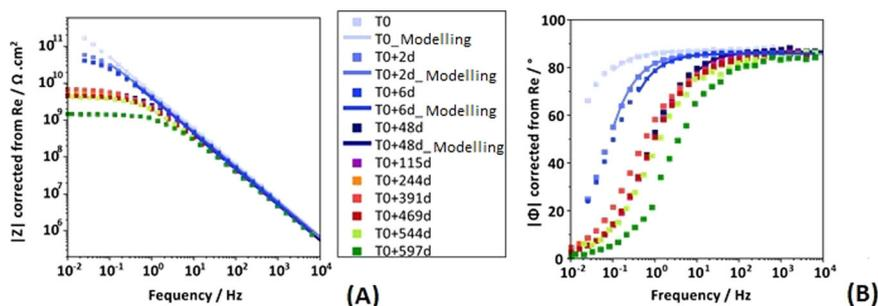
**Fig. 4** Bode diagrams obtained regularly during 597 days of painted DH36 steel immersed in seawater. The modulus in (A) and phase in (B) are plotted as a function of frequency, in artificial seawater at 20 °C, under natural aeration and static conditions.
