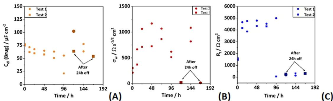
**Fig. 14** Progression of the EEC parameters during the 7 days of cathodic polarization with two days of interruption (the 5th and 7th days). The double layer capacitance (Cdl) estimated with Brug's law in (A), the Warburg constant for the diffusion phenomenon ( $\sigma_w$ ) in (B), and the charge transfer resistance ( $R_{ct}$ ) or the faradic impedance ( $Z_f$ ) in (C), for an unpainted DH36 steel immersed for 7 days in a naturally aerated solution, in a static condition at 20 °C.
