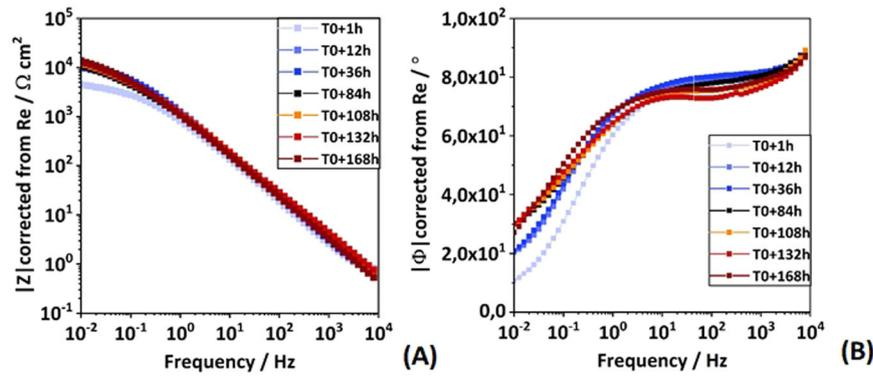
**Fig. 8** Bode diagrams measured regularly during 7 days of continuous cathodic polarization at  $-0.8$  V vs SCE of DH36 steel. The modulus in (A) and phase in (B) are plotted in function of the frequency and corrected for Re (electrolyte resistance). Measurements are made after 1 h, 12 h, 36 h, 84 h, 108 h, 132 h, and 168 h of immersion at  $20$  °C, under static condition and natural aeration.
