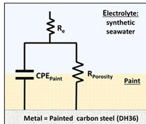
**Fig. 3** Equivalent Electrical Circuit (EEC) of a freshly painted steel/seawater interface. It illustrates the case of a freshly painted, defect-free sample immersed in seawater after 2 h at OCP (Open Circuit Potential), at 20 °C in static condition and natural aeration.
