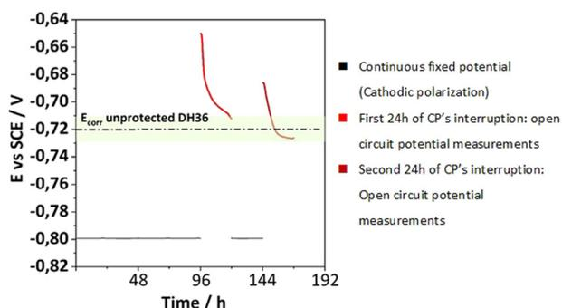
**Fig. 15** Monitoring of the potential at the DH36 surface under on/off period of cathodic protection. Potential at DH36 surface in the function of the time, at 20 °C, static conditions and in natural aeration condition.
