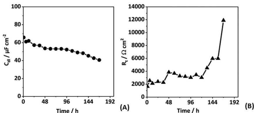
**Fig. 11 EEC model parameters evolution during the 7 days of continuous cathodic polarization.** Double-layer capacitance ( $C_{dl}$ ) estimated with the Brug law's in (A) and a charge transfer resistance ( $R_t$ ) in (B) in function of time and estimated from EIS data measured with EC-LAB® software modelling, in static conditions, natural aeration, and 20 °C.
