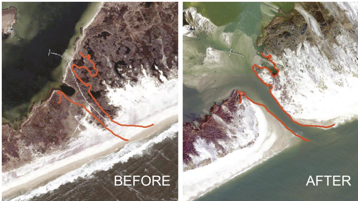
2 Fig. 2 Photos before and after Hurricane Sandy (2012) opened a breach on Fire Island, and created a washover deposit behind the dune barrier 3 (USGS Public Domain)
