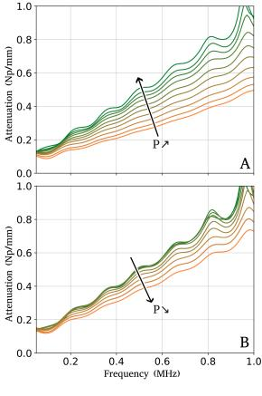
Figure 4. Evolution of the (longitudinal-wave) attenuation for the sample containing the micro-balloons, as a function of frequency for different static loads. The applied pressure increases from 1 to 10 bars by steps of 1 bar (A), and decreases down to 1 bar with the same steps (B).
