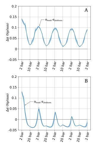
Figure 5. Evolution of the attenuation difference  $\Delta \alpha$  =  $\alpha_{\rm beads} - \alpha_{\mu - \rm balloons}$  measured at 50 kHz over 4 cycles of compression/relaxation for applied pressure ranging from 2 bars up to 10 bars (A) or to 20 bars (B). The areas represent the repeatability of the experiments and the solid line corresponds to the mean value.
