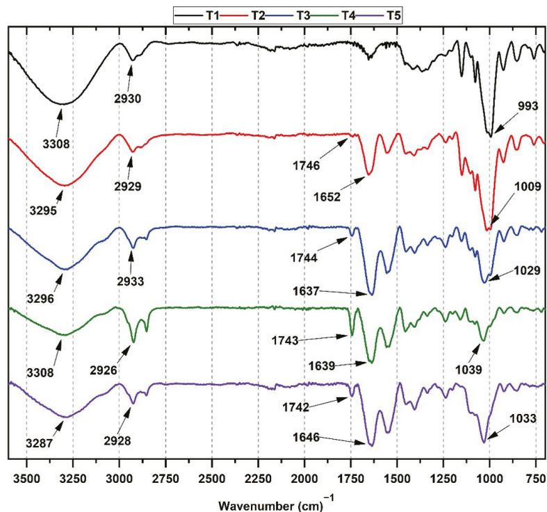
**Figure 1.** FTIR spectra of cassava starch/gelatin films. T1 gelatin/cassava starch 0/100; T2 gelatin/cassava starch 25/75; T3 gelatin/cassava starch 50/50; T4 gelatin/cassava starch 75/25; T5, gelatin/cassava starch 100/0.
