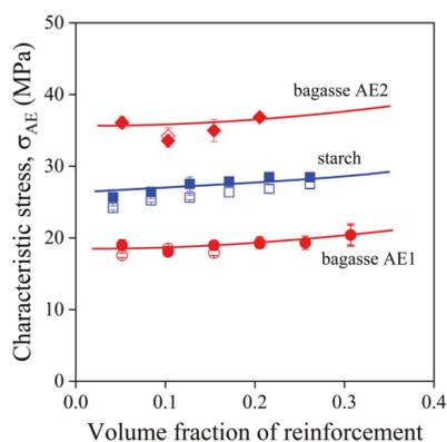
**Figure 7.** Composition dependence of characteristic stresses derived from acoustic emission testing. Symbols: (○, ●) sugarcane bagasse fibers,  $\sigma_{AE1}$  (□, ■) starch,  $\sigma_{AE}$  (◇, ◆) bagasse,  $\sigma_{AE2}$ ; empty symbols without MAPLA, full symbols with MAPLA.
