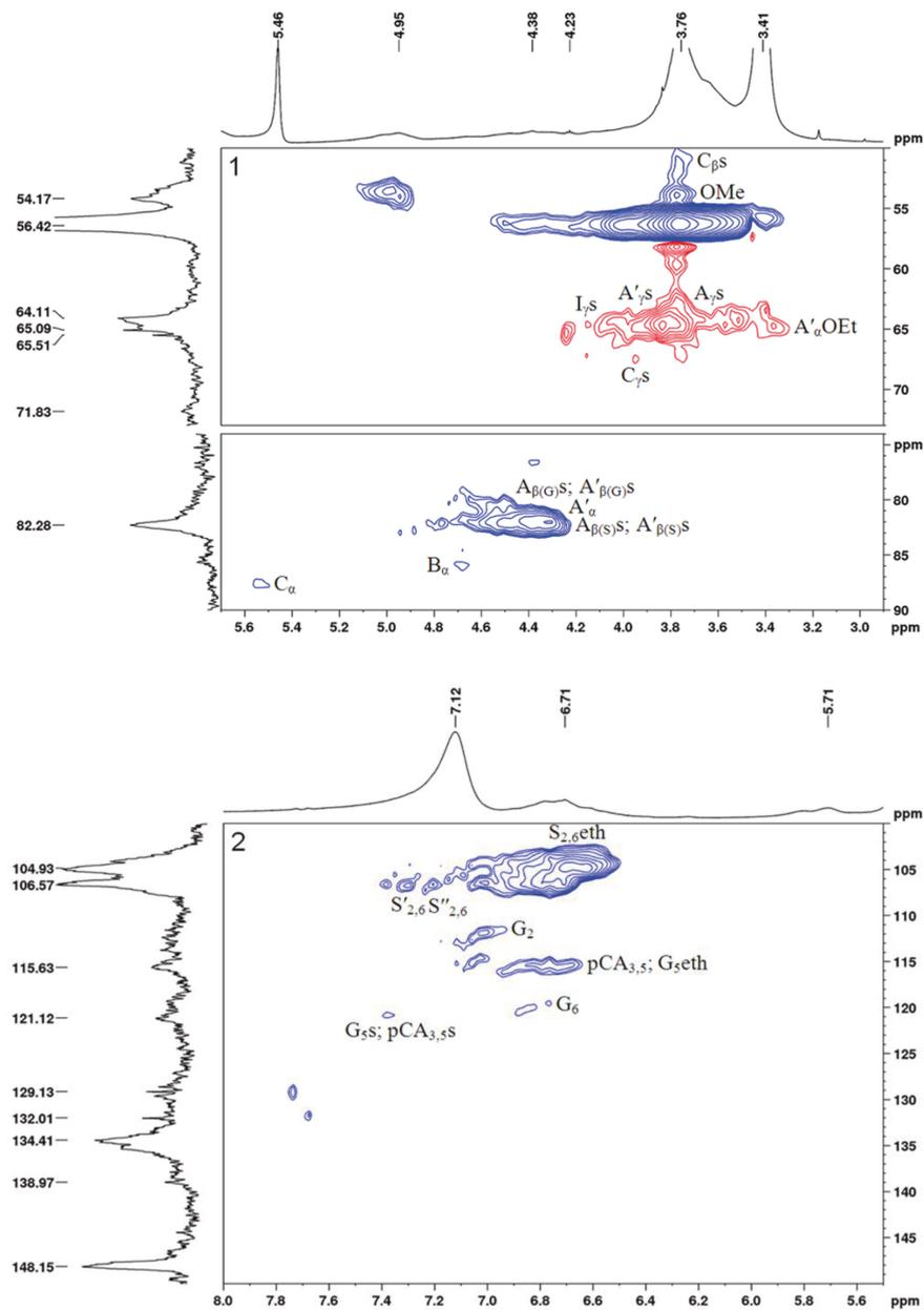
**Figure 10.** HSQCed spectrum of sulfated ethanol lignin: aliphatic oxygenated region 1 and aromatic region 2. The assignment of signals is given in Table 5, and the main identified structural units and fragments are shown in Figure 11.
