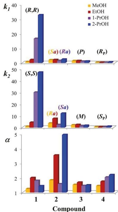
**Figure 2.** Effect of mobile phase on the retention ( $k_1$  and  $k_2$ ) and enantioselectivity ( $\alpha$ ) factors of 1–4. Chromatographic conditions: column, Chiralpak AD-3 (100 mm  $\times$  4.6 mm, 3  $\mu$ m); flow rate, 1 mL/min; temperature, 25  $^{\circ}$ C; detection, UV and CD at 241 nm. 2-PrOH: 2-propanol; 1-PrOH: 1-propanol, EtOH: ethanol; MeOH: methanol.
