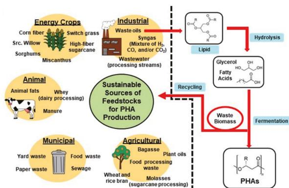
**Figure 7.** Sustainable sources and conversion of feedstocks for PHA production. Provided within the dashed area is a simplified representation of the conversion of waste oils (lipids) to PHAs. The waste lipid is hydrolyzed to yield substrates for fermentation: fatty acids and glycerol. The substrates are purified prior to use in fermentations. Recovered waste biomass can be recycled as a carbon source for future fermentations.
