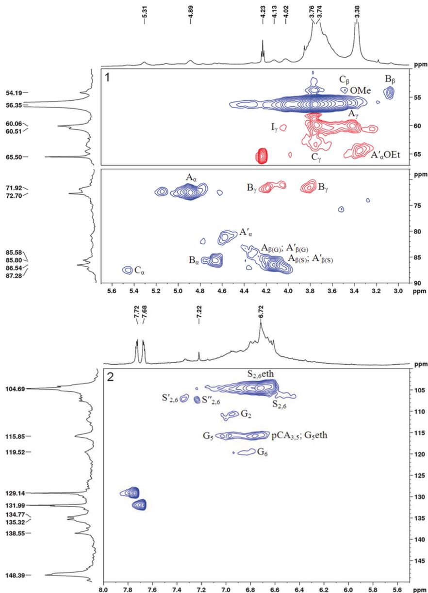
**Figure 9.** HSQCed spectrum of ethanol lignin: aliphatic oxygenated region 1 and aromatic region 2. The assignment of signals is given in Table 5, and the main identified structural units and fragments are shown in Figure 11.
