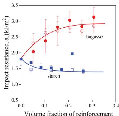
**Figure 4.** Dependence of the notched Charpy impact resistance of PLA composites containing natural reinforcements. Symbols: (○, ●) sugarcane bagasse fibers, (□, ■) starch; empty symbols without MAPLA, full symbols with MAPLA.
