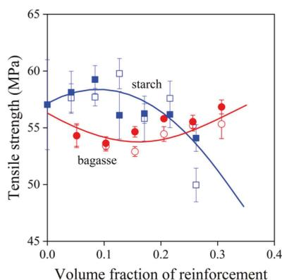
**Figure 3.** Effect of composition and coupling on the tensile strength of PLA composites. Symbols: (○, ●) sugarcane bagasse fibers, (□, ■) starch; empty symbols without MAPLA, full symbols with MAPLA.
