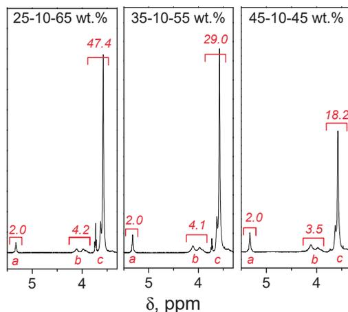
**Figure 1.**  $^1\text{H}$  NMR spectra of terpolymers HOSBM-BA-MMA.
