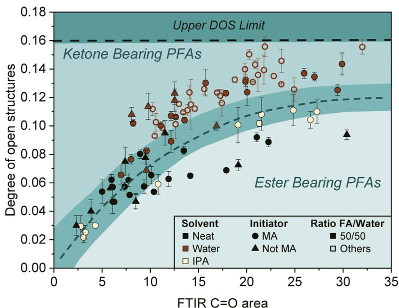
**Figure 5.** Degree of open structures obtained with titration method against FTIR C=O area for PFA synthesized in neat, aqueous and 50/50 IPA systems. PFA have been synthesized with aforementioned catalysts.
