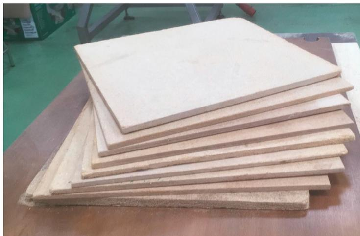
Figure 4. Samples of the experimental particleboards.
