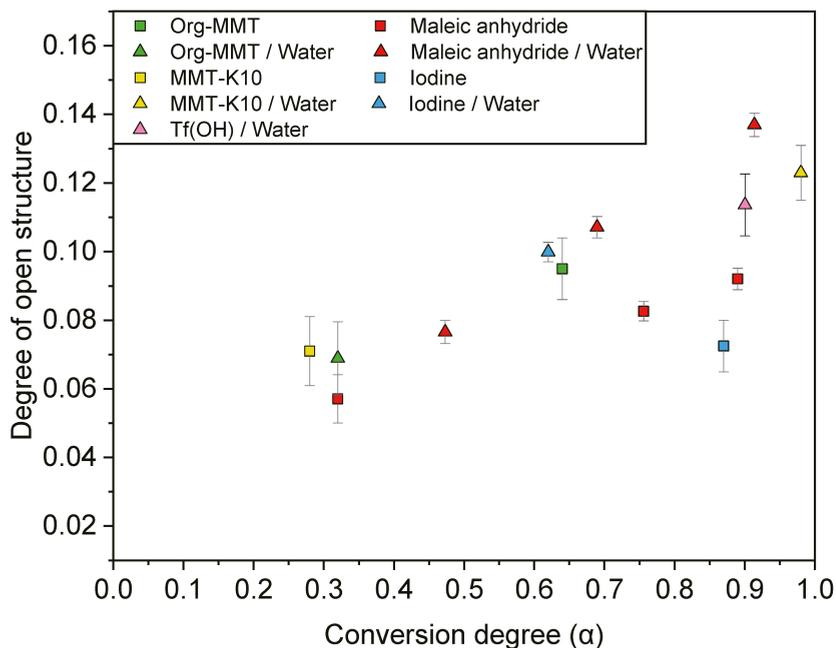
**Figure 2.** Comparison of the degree of open structures obtained by titration method and synthesized with different initiators with and without additional water (50/50 *w/w*) as function of the conversion degree.
