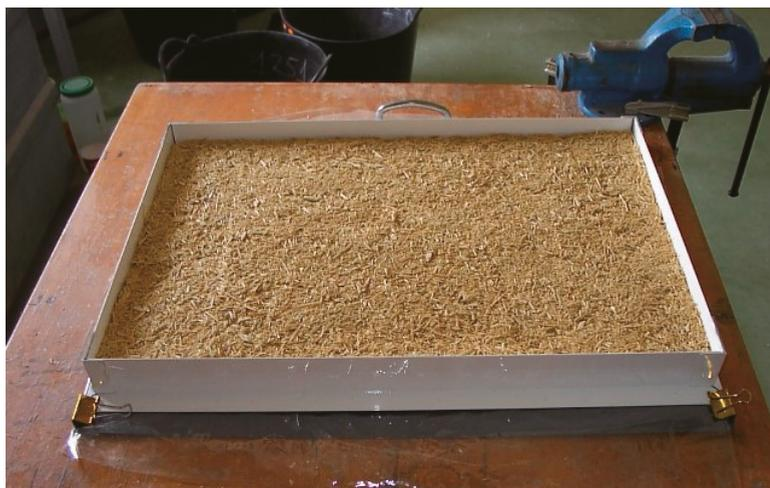
Figure 3. Mat formed manually to manufacture the particleboards.
