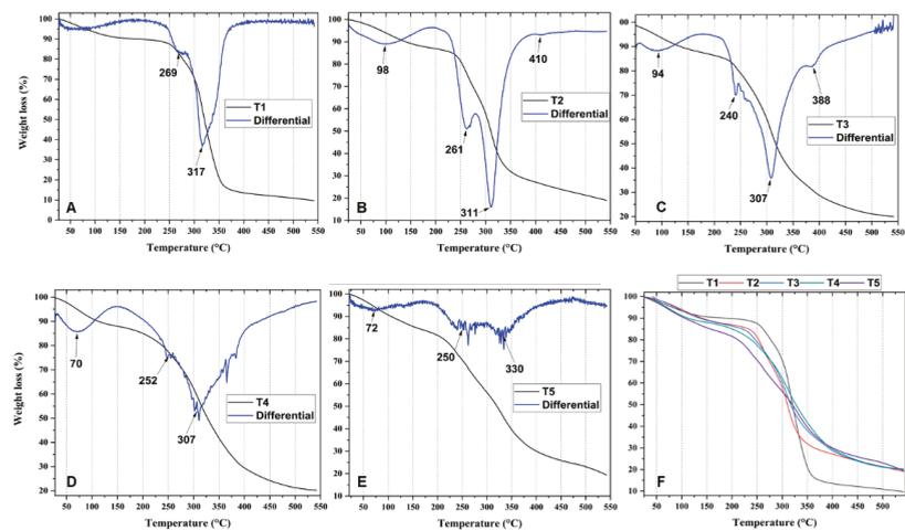
**Figure 2.** Thermogravimetric analysis for T1, (A) gelatin/cassava starch 0/100; T2, (B) gelatin/cassava starch 25/75; T3, (C) gelatin/cassava starch 50/50; T4, (D) gelatin/cassava starch 75/25; T5, (E) gelatin/cassava starch 100/0; (F) All the samples.
