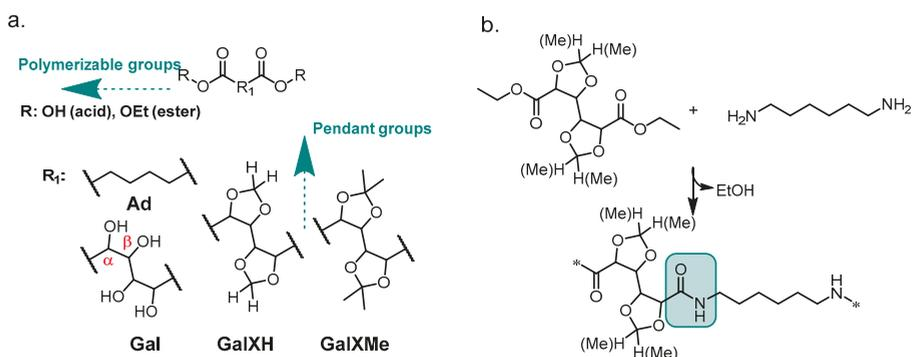
**Figure 1.** (a) The general structure of the investigated acetals (GalXH and GalXMe) and adipate motif (Ad); (b) the polymer obtained by reacting diethyl esters of GalXH and GalXMe with 1,6-hexamethylenediamine.
