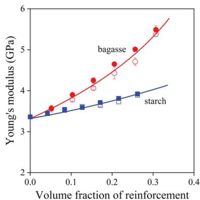
**Figure 2.** Composition dependence of the stiffness of PLA composites reinforced with starch or bagasse fibers. Effect of coupling. Symbols: (○, ●) sugarcane bagasse fibers, (□, ■) starch; empty symbols without MAPLA, full symbols with MAPLA.
