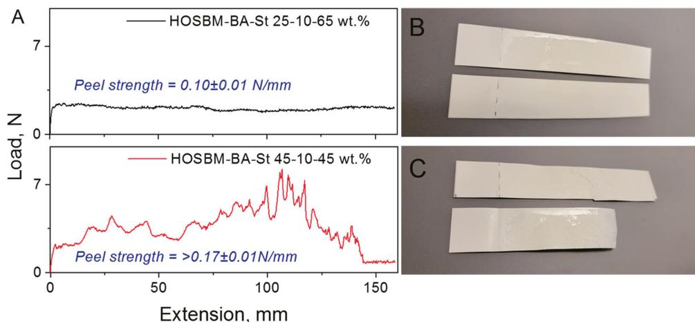
**Figure 6.** Peel strength of HOSBM-BA-St 25–10–65 wt. % and 45–10–45 wt. % latexes copolymers on paperboard (coated to uncoated) substrates (A) and substrate samples after peel strength testing ((B,C) [substrate failure]).
