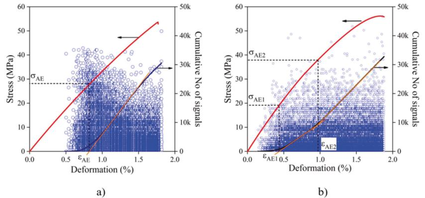
**Figure 6.** Results of the acoustic emission testing of PLA composites containing starch or bagasse fibers. Additive content: 20 vol%. Symbols: (○) individual acoustic events, full lines: stress vs. deformation (left axis, red) and cumulative number of signal vs. deformation (right axis, navy) correlations: (a) starch, (b) sugarcane bagasse fiber.
