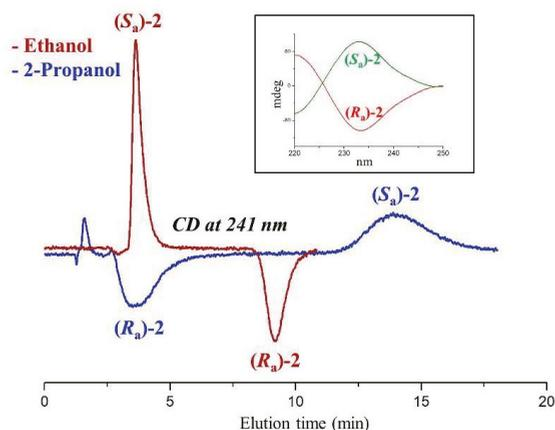
**Figure 3.** Typical chromatograms illustrating the differences in enantiomer elution order of **2** using pure ethanol and 2-propanol as mobile phases. Chromatographic conditions: column, Chiralpak AD-3 (100 mm × 4.6 mm, 3 μm); flow rate, 1 mL/min; temperature, 25 °C; detection, CD at 241 nm. 2-PrOH: 2-propanol; 1-PrOH: 1-propanol, EtOH: ethanol; MeOH: methanol. Inset: CD spectra of enantiomers of **2**.
