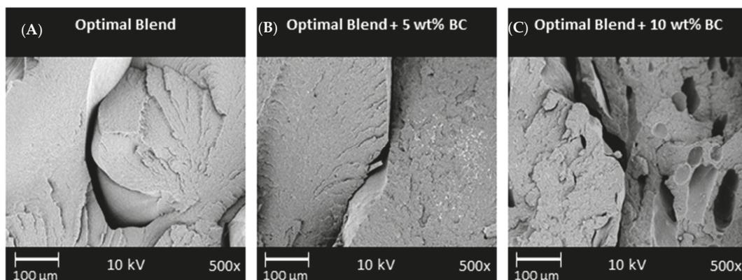
**Figure 6.** SEM images of the impact fracture surface for FFF samples for the (A) optimal polymer blend, (B) optimal blend with 5 wt % biocarbon, and (C) optimal blend with 10 wt % biocarbon. See Table 2 for nomenclature for optimal blend.
