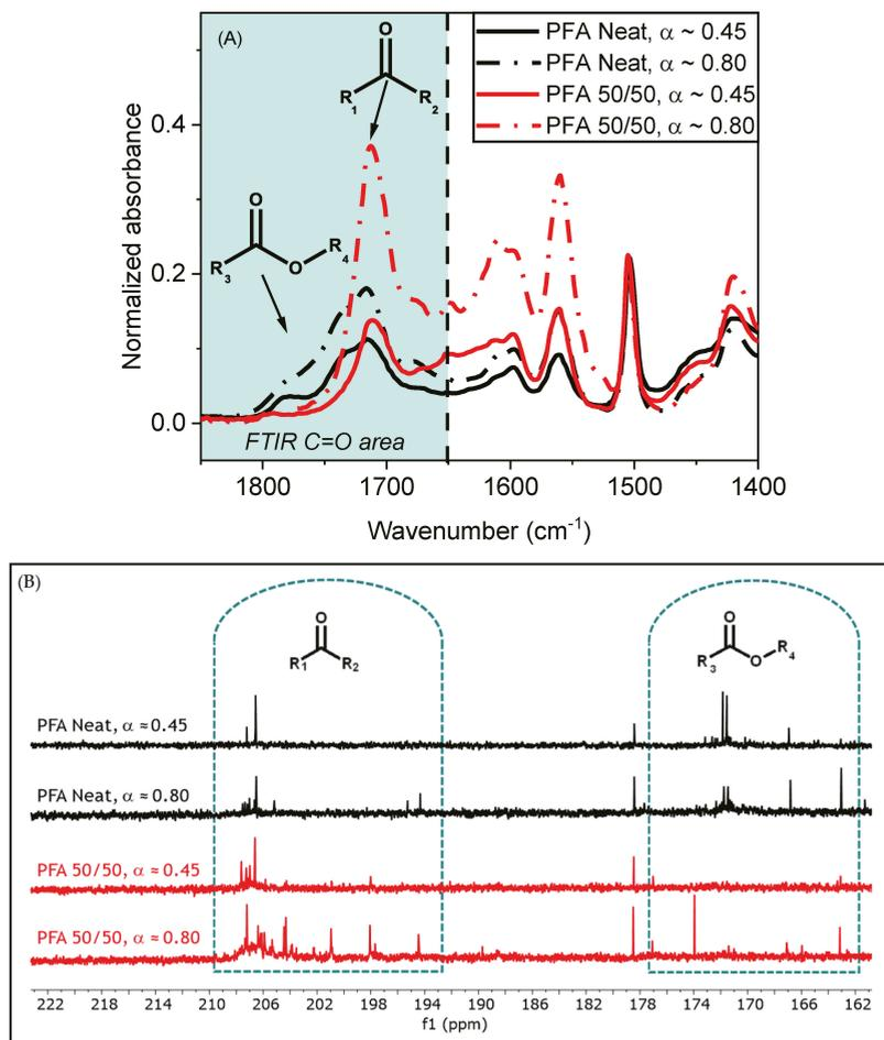
**Figure 4.** (A) Normalized FTIR spectra of PFA 50/50 water and neat PFA neat at  $\alpha \approx 0.5$  and  $\alpha \approx 0.8$ . (B)  $^{13}\text{C}$  NMR spectra of PFA 50/50 water and neat PFA at  $\alpha \approx 0.5$  and  $\alpha \approx 0.8$  with an accumulation of 6000 scans.
