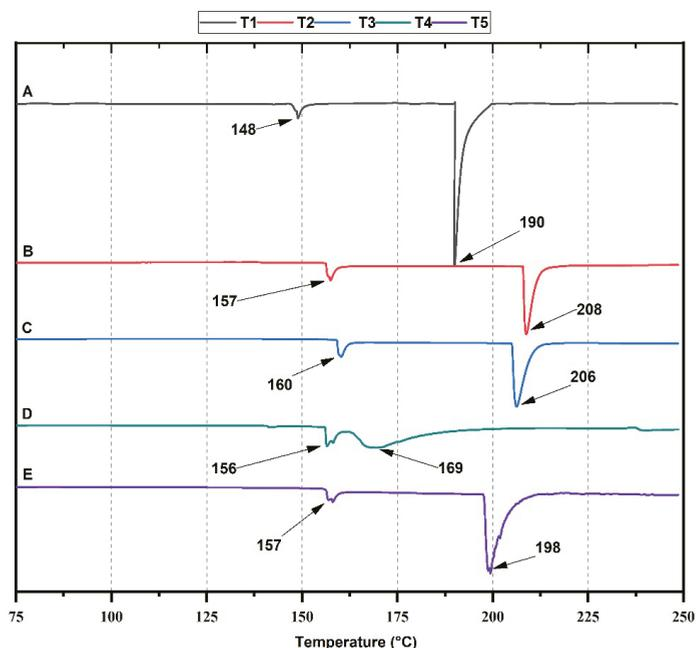
**Figure 3.** DSC thermogram of films: T1, (A) gelatin/cassava starch 0/100; T2, (B) gelatin/cassava starch 25/75; T3, (C) gelatin/cassava starch 50/50; T4, (D) gelatin/cassava starch 75/25; T5, (E) gelatin/cassava starch 100/0.
