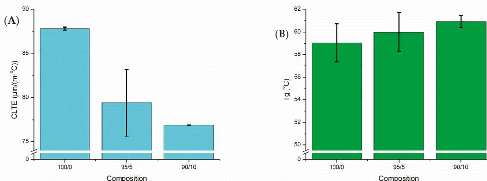
**Figure 4.** Thermomechanical analysis of the blend and composites: (A) coefficient of linear thermal expansion (CLTE) and (B) glass transition temperature ( $T_g$ ) where injection molded samples were used. See Table 2 for nomenclature.
