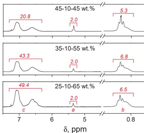
**Figure 2.**  $^1\text{H}$  NMR spectra of terpolymers HOSBM-BA-St.
