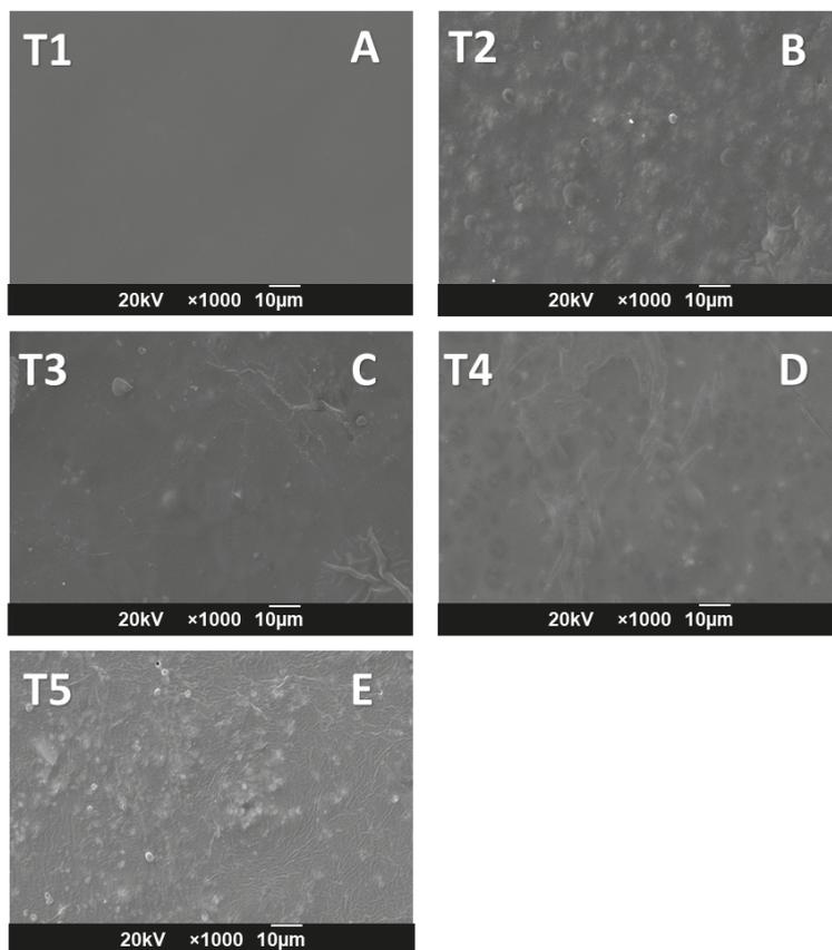
**Figure 4.** Morphological analysis of slides by scanning electron microscopy (SEM): T1, (A) gelatin/cassava starch 0:100; T2, (B) gelatin/cassava starch 25/75; T3, (C) gelatin/cassava starch 50/50; T4, (D) gelatin/cassava starch 75/25; T5, (E) gelatin/cassava starch 100/0.
