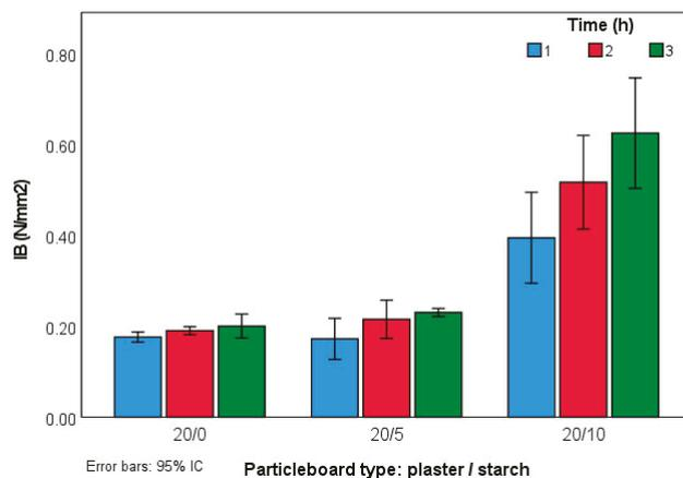
Figure 7. IB values of the experimental panels.
