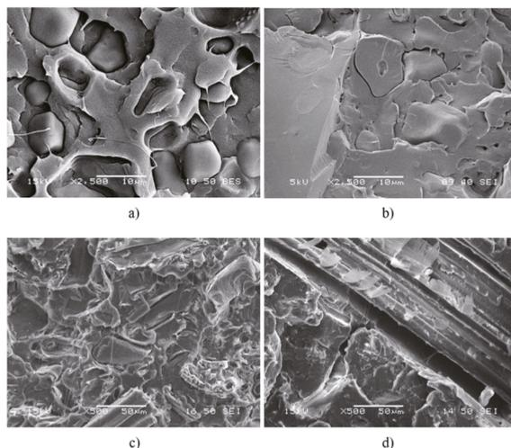
**Figure 8.** SEM micrographs recorded on the fractured surfaces of specimens broken during tensile testing: (a) starch, 20 wt%; (b) starch, 20 wt%, MAPLA; (c) sugarcane bagasse fiber, 20 wt%; and (d) bagasse fiber, 20 wt%, MAPLA.
