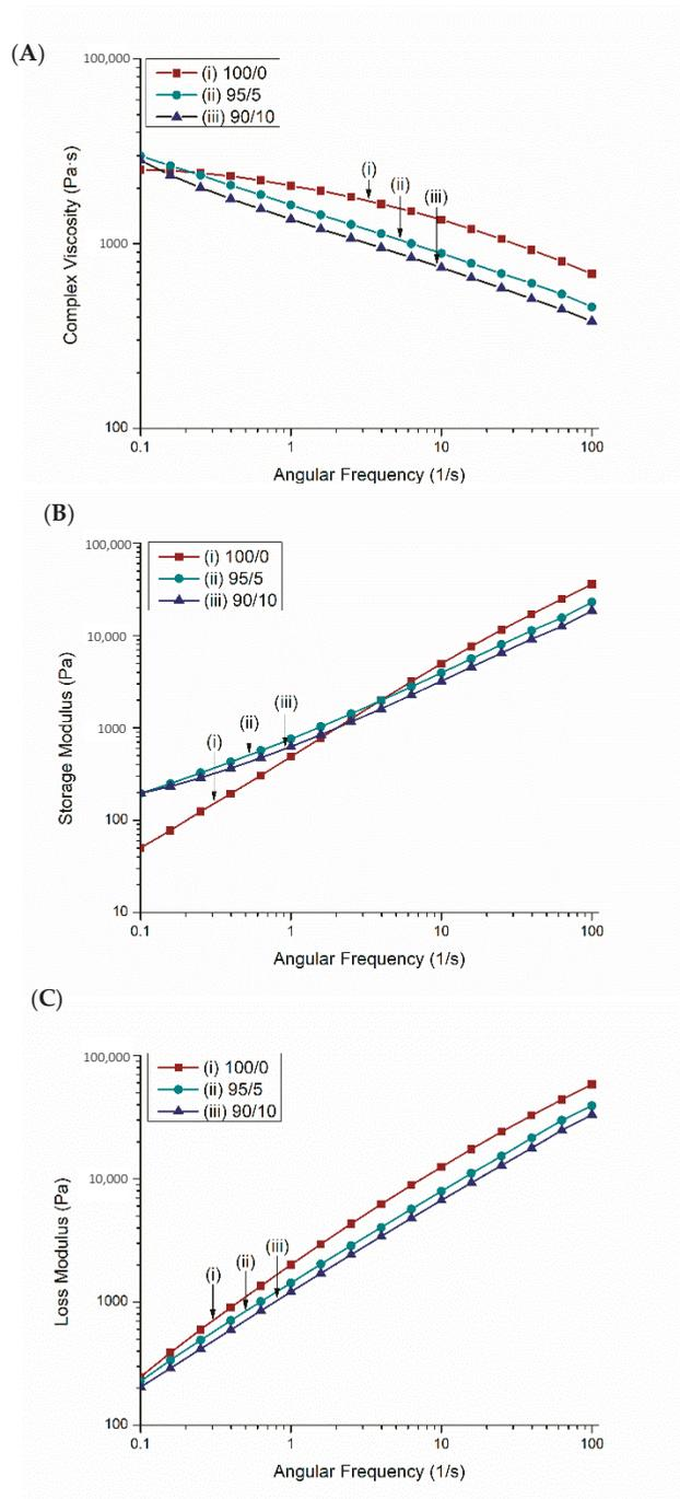
**Figure 5.** Rheological analysis of composites: (A) complex viscosity ( $\eta$ ), (B) storage modulus ( $G'$ ), and (C) loss modulus ( $G''$ ) for injection molded samples of the PTT blend and *Miscanthus* BC composites. See Table 2 for nomenclature.
