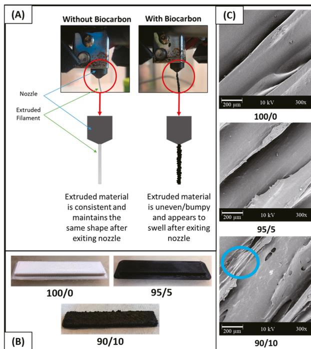
**Figure 2.** PTT/BC biocomposites in FFF: (A) the upper left section provides a comparison of an extrudate with and without biocarbon to depict challenges with consistency, (B) the lower left section compares FFF samples with different BC content for surface roughness, and (C) the right side of the image examines SEM images of the FFF surface of FFF printed samples. See Table 2 for nomenclature.
