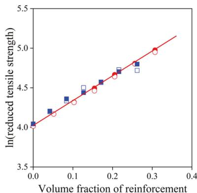
**Figure 5.** Reinforcing effect of the natural additives used in PLA composites. Tensile strength plotted in the linear representation of Equation (2). Effect of coupling. Symbols: (○, ●) sugarcane bagasse fibers, (□, ■) starch; empty symbols without MAPLA, full symbols with MAPLA.
