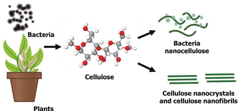
Figure 1. Formation of nanocellulose from cellulose-containing materials.
