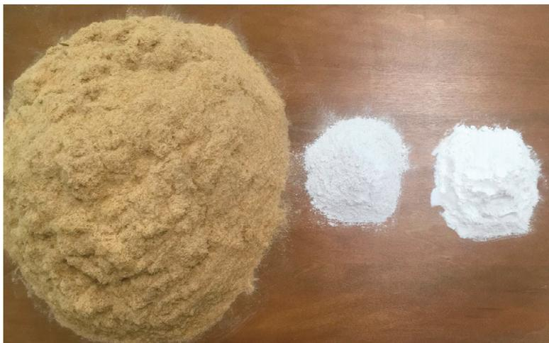
**Figure 2.** Giant reed (left), gypsum (center), and starch (right) particles used for manufacturing the experimental board type 20:10.
