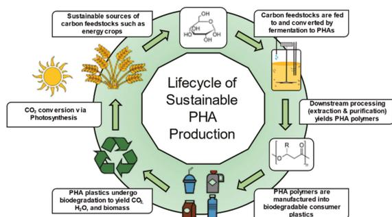
**Figure 3.** Using renewable, low-cost carbon sources such as energy crops or waste streams in combination with optimized fermentation strategies supports high yielding PHA production processes. The PHA polymers are processed and manufactured into consumer plastics that will biodegrade when disposed. The cycle begins again when biodegradation products of PHA plastics are consumed during photosynthesis or are recovered in waste streams from composting facilities.
