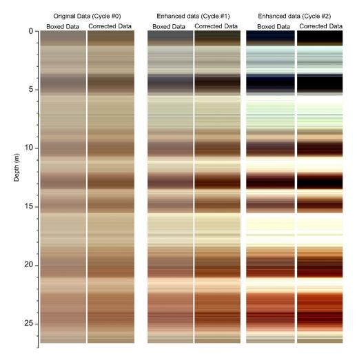
**Fig. 5.** Compares the applied colorimetric enhancement cycles performed on the SK18 LPS (1336 samples) boxed material before and after correction. Note that the original data of the uncorrected box material (leftmost panel) are RGB values calculated from the average L\*, a\*, and b\* values of 5 measured DRS-spectra for each of the 1336 samples (i.e., a total of 6680 individual DRS-spectra measurement).
