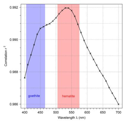
Fig. 3. Compilation of correlation coefficients for each wavelength. Wavelength intervals from which goethite and hematite TBA are extracted are highlighted in blue and red.
