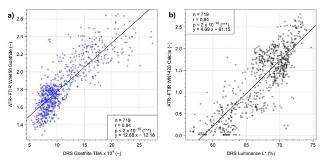
**Fig. 6.** a) Comparison of DRS-derived qualitative goethite content from corrected box data and ATR-FTIR-derived goethite content. b) Comparison of DRS-derived L<sup>\*</sup> values from corrected box data, considered here as a proxy of calcite content (see text), and ATR-FTIR-derived calcite content. Based on 719 data points, both comparisons follow a linear trend and correlate significantly well.
