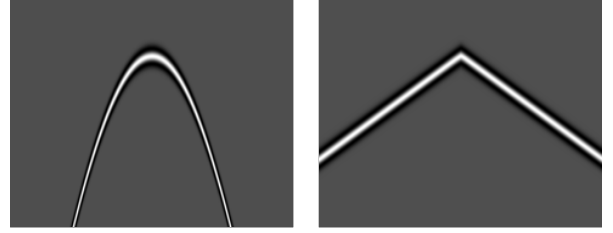
Fig. 2: Two elements of the dictionary developed in [35]: the left one has a correct shape whereas the right one is an outlier.
