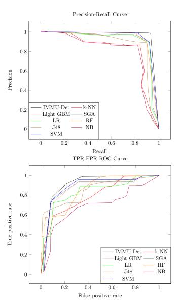
Fig. 4. IMMU-Det's obtained ROC curves with different classifiers.
