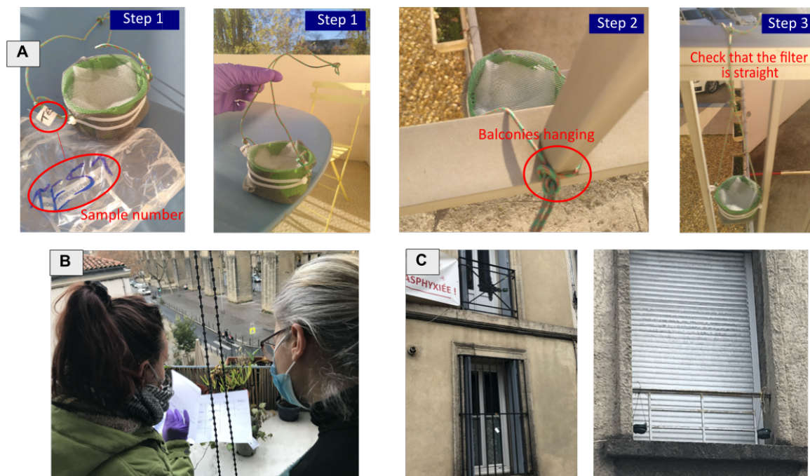
Figure 3: [a] Extract from the protocol designed to facilitate the deposimeters set up by the inhabitants. [b] Protocol presentation and explanation during the kit distribution. [c] Examples of the settled filters pictures sent by citizen partners.
