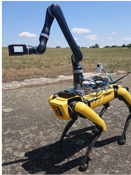
Figure 1: The Spot ® quadruped robot, mounted with extra payload. The controller code was generated from a skillset which was verified a-priori with SkiNet. The skillset in Fig 2 is an extract of the actual running skillset, available at https://gitlab.com/onera-robot-skills/skinet-release .
