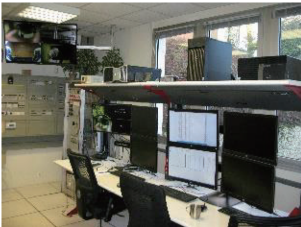
Fig.6. The new control room (since 2021). The centrifuge parameters are controlled on the computer, the former board being only maintained for decorating (top) and the tests parameters (jacks, data acquisition system...) are controlled and recorded on several screens and computers (bottom).
