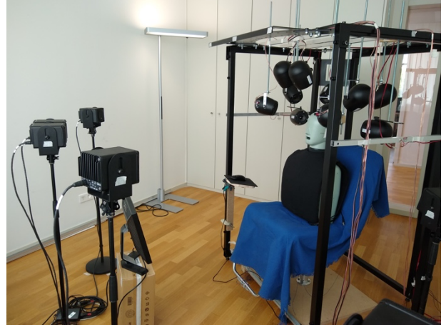
Fig. 5. Experimental setup. On the right of the seat, a mouse allows usage of the test interface displayed on the screen placed in front of the listener.
