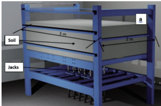
Fig.6. The Ineris device for simulating underground movements, controlled by a set of jacks located under the soil (Al Heib et al., 2020, 2021).
