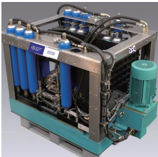
Fig.11. 1D earthquake simulator (from Chazelas et al., 2008).
