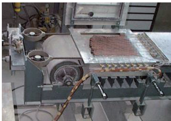
Fig. 3. Base-friction table in EPF Lausanne, Switzerland (courtesy from P. Egger).
