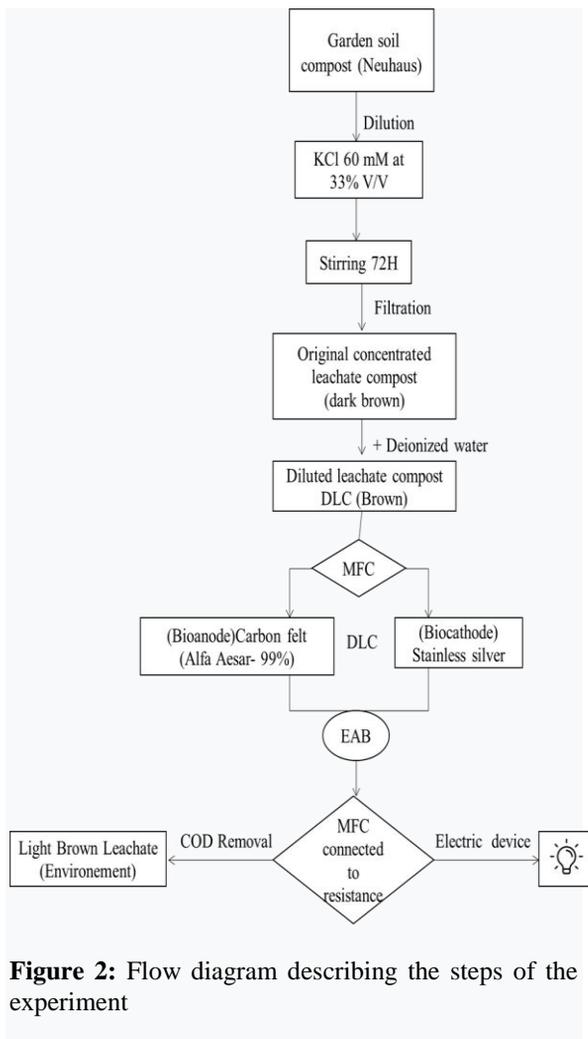
**Figure 2:** Flow diagram describing the steps of the experiment
