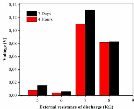
**Figure 3:** Evolution curves of MFCs discharging into the polarizing electric resistances 5, 6, 7 and 8 kΩ, successively during the 1<sup>st</sup> day (during 4 h) and at the end of the experiment (7<sup>th</sup> day).
