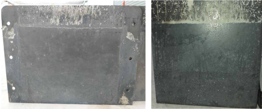
387 Fig. 8. Surface condition of the molds after stripping: VO on the left, Hc-2 on the right
