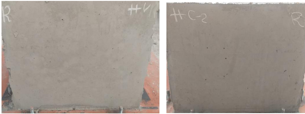
Fig. 10. Concrete facing obtained after 7 days: VO on the left, Hc-2 on the right
