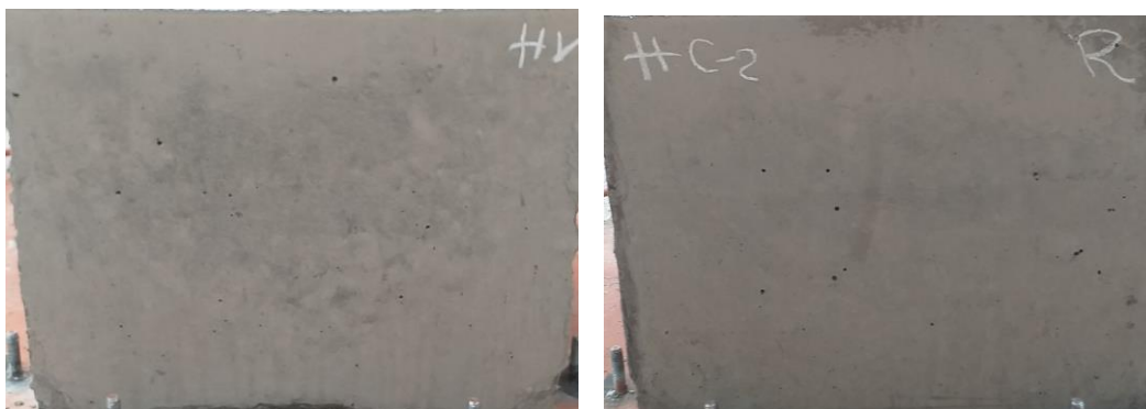
396 Fig. 9. Concrete facing obtained after 1 day: VO on the left, Hc-2 on the right
