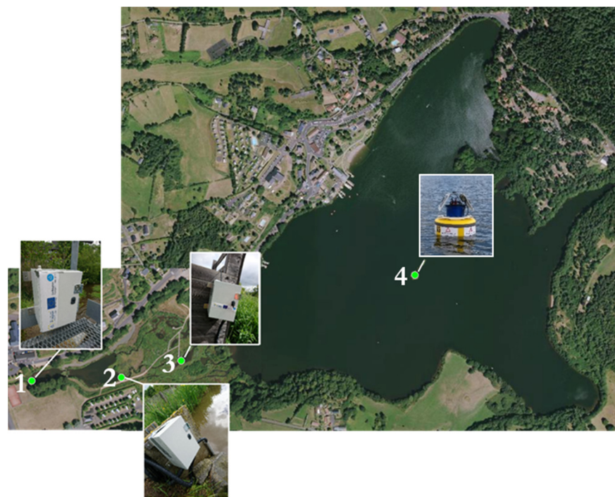
Figure 7. Location of sensors on Aydat site (1, 2, and 3: Aquatroll 200 data logger, 4: Hydrolab HL7) (Image ©2023 Google, Images ©2023 CNES/Airbus).
