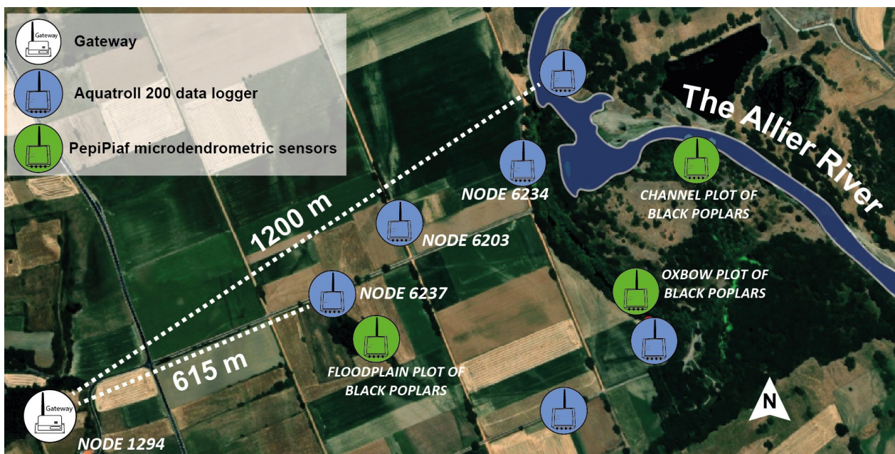
Figure 8. Location of sensors on the Auzon site (Image ©2023 Google, Images ©2023 CNES/Airbus).
