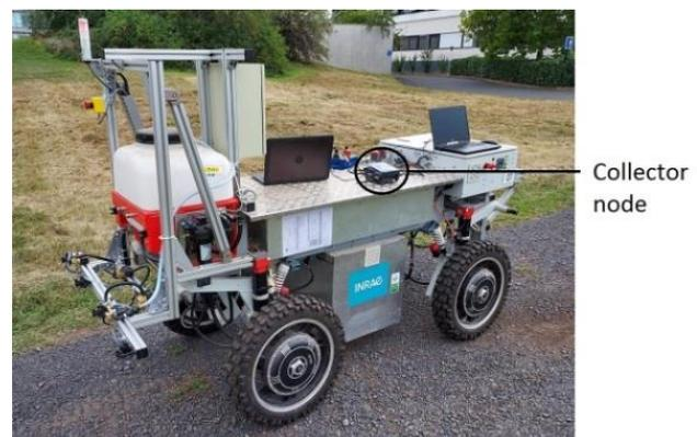
Figure 9. Experimental robot used for the tests
