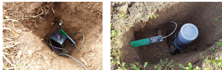
Figure 1. Examples of sensor nodes buried at 15 cm from the surface in a pasture with a moisture probe on the side [12]. The nodes will next be covered with soil and compacted.
