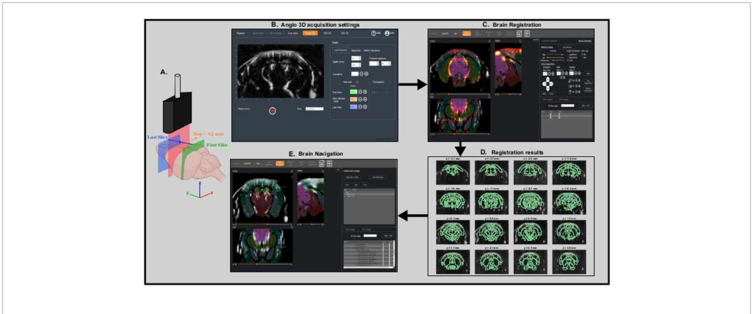
Figure 3: Fast transcranial angiographic Scan and Brain registration for precise probe positioning. A. Schematic representation of the mouse brain being scanned transcranially by the ultrasonic probe from the first coronal slice (green) to the last coronal slice (blue) during a fast angiographic scan. The current imaged slice (represented in red) moves step by step from the back (green) to the front (blue) of the brain. Created with BioRender.com B. Screenshot of IcoScan acquisition software in the Angio 3D panel. The preset parameters on the right configure the fast scan. The positions in mm of the first slice, the last slice and the step size must be well chosen to scan linearly the whole brain. C. Screenshot of the IcoStudio processing software. The fast Angio 3D scan is automatically registered to a reference template of the mouse brain. The three-views (left) shows the superposition of the vasculature and the mouse brain Allen atlas in the coronal, sagittal and axial views. D. Linear lay-out (montage) of 16 slices (out of 31) from the 3D angio scan, with the registered Allen reference atlas superimposed onto the vasculature. E. Screenshot of the Brain Navigation panel showing the predicted imaging plane corresponding to the motor coordinates computed by the software thanks to the two markers placed at the center of the left and right primary somatosensory cortex, barrel fields region. Please click here to view a larger version of this figure.
