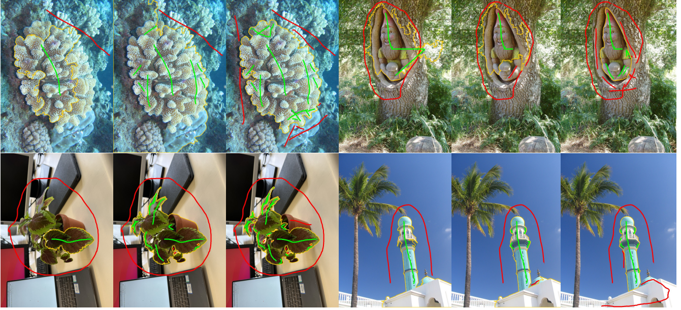
Fig. 4. Three stages in an interactive segmentation session. The red lines represent background seeds, the green lines represent object seeds, and the yellow lines represent the segmentation produced by the current set of seeds.
