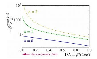
FIG. 7. The first three nonzero coefficients in the series (88) of the free energy of the ring as a function of the (inverse) normalized radius 1/L. The direction of the thermodynamic limit is shown by the arrow.
