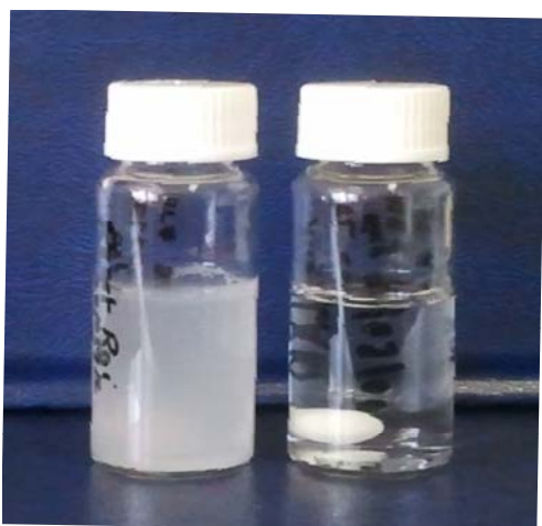
Fig. S11. Photograph of gellan gum samples after stirring for 1 hour in 80°C water: high-acyl gellan (left) and low-acyl gellan (right). Both samples contain a white oval magnetic stirrer, clearly visible in right vial and hardly discernable in the left vial.
