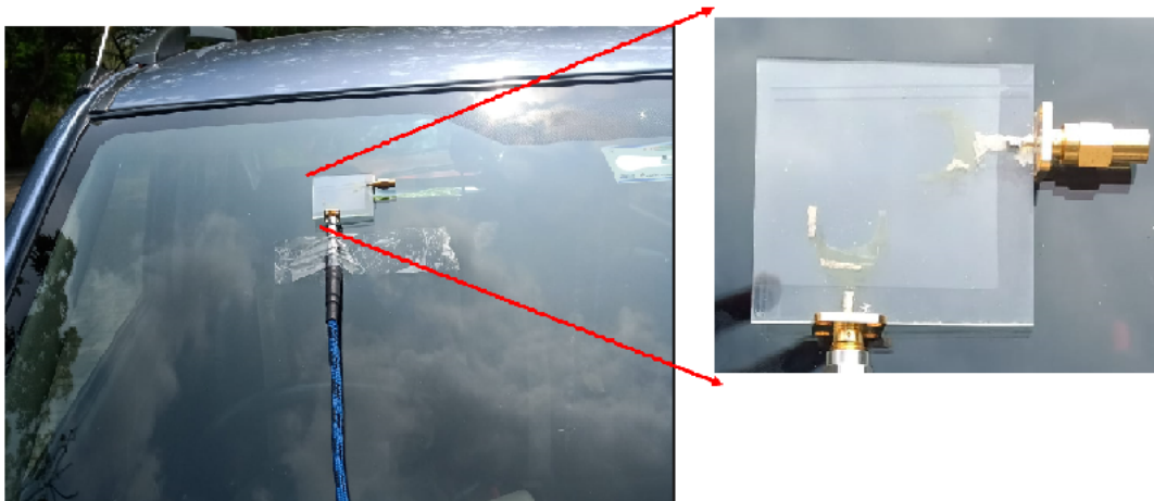
Figure 7. Fabricated prototype of the MIMO antenna
