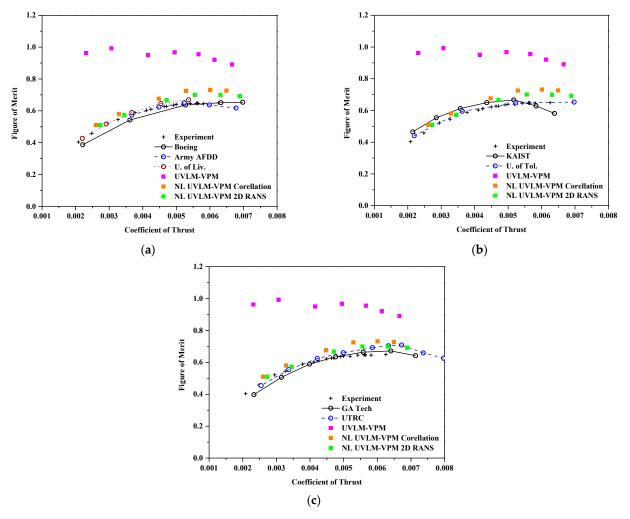
**Figure 8.** Figure of merit with coefficient of thrust C<sub>T</sub>, comparisons between hybrid UVLM-VPM and experimental data with (**a**) 3D RANS structured codes, (**b**) 3D RANS/DES unstructured codes, and (**c**) hybrid 3D RANS-Lagrangian codes.
