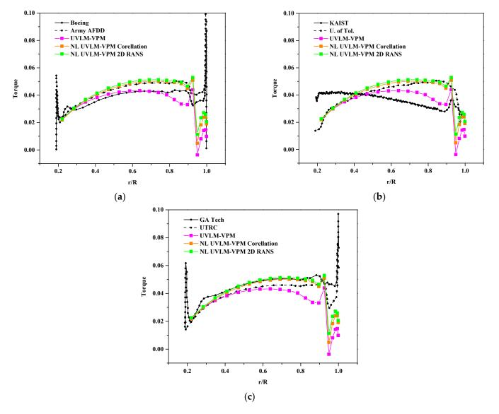
**Figure 10.** Blade section torque coefficient  $C_q$  for  $C_T/\sigma = 0.09$ , comparisons between hybrid UVLM-VPM with (**a**) 3D RANS structured codes, (**b**) 3D RANS/DES unstructured codes, and (**c**) hybrid 3D RANS-Lagrangian codes.
