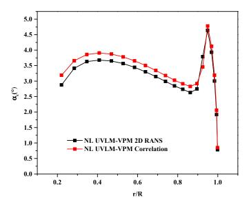
**Figure 5.** Effective angle of attack distribution along the span at a collective angle of 9.25° and tip Mach number of 0.65 out of ground effect using the RANS database in black and Bousman experimental correlation in red.
