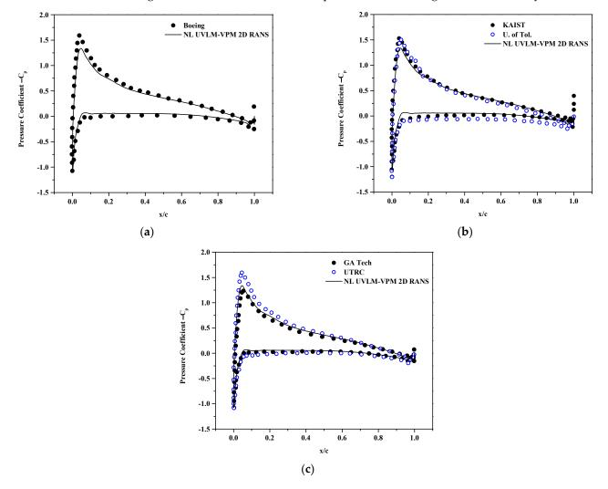
**Figure 12.** Surface pressure coefficient  $-C_p$  at r = 0.85R and  $C_T/\sigma = 0.09$ , comparisons between hybrid UVLM-VPM with (a) 3D RANS structured codes, (b) 3D RANS/DES unstructured codes, and (c) hybrid 3D RANS-Lagrangian codes.
