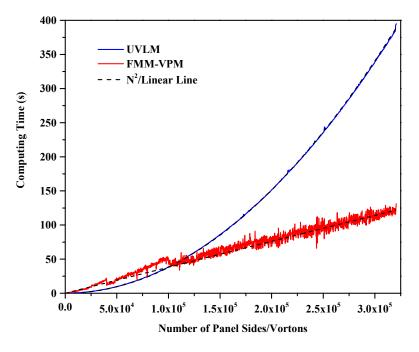
Figure 2. Time for wake evolution steps versus the number of elements for direct UVLM and FMM VPM.
