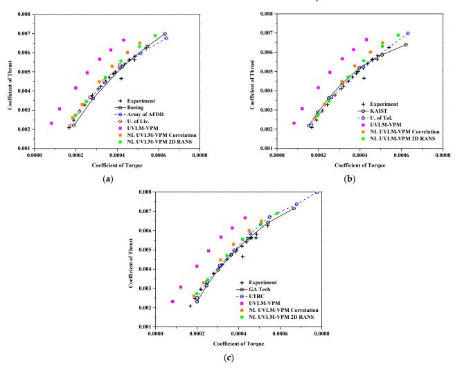
**Figure 7.** Coefficient of thrust  $C_T$  varying with coefficient of torque  $C_Q$ , comparisons between hybrid UVLM-VPM and experimental data with (**a**) 3D RANS structured codes, (**b**) 3D RANS/DES unstructured codes, and (**c**) hybrid 3D RANS-Lagrangian codes.
