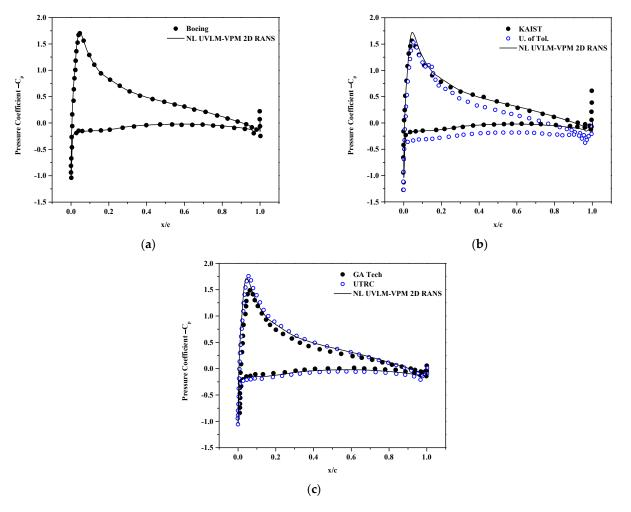
**Figure 11.** Surface pressure coefficient  $-C_p$  at r = 0.6R and  $C_T/\sigma = 0.09$ , comparisons between hybrid UVLM-VPM with (**a**) 3D RANS structured codes, (**b**) 3D RANS/DES unstructured codes, and (**c**) hybrid 3D RANS-Lagrangian codes.
