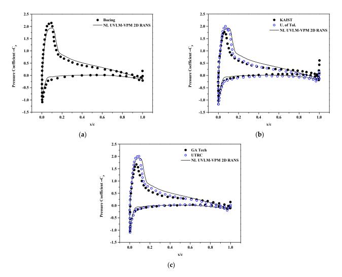
**Figure 13.** Surface pressure coefficient  $-C_p$  at r = 0.975R and  $C_T/\sigma = 0.09$ , comparisons between hybrid UVLM-VPM with (**a**) 3D RANS structured codes, (**b**) 3D RANS/DES unstructured codes, and (**c**) hybrid 3D RANS-Lagrangian codes.
