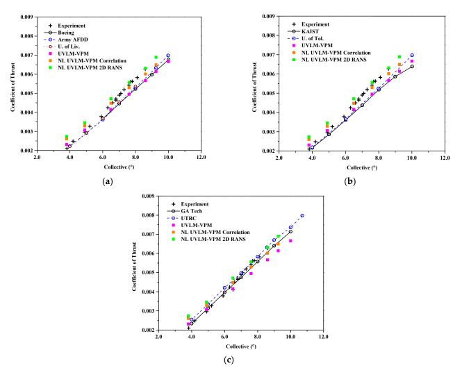
**Figure 6.** Coefficient of thrust  $C_T$  varying with collective angle, comparisons between Hybrid UVLM-VPM and experimental data with (**a**) 3D RANS structured codes, (**b**) 3D RANS/DES unstructured codes, and (**c**) hybrid 3D RANS-Lagrangian codes.
