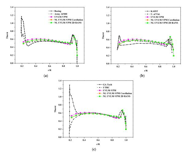
**Figure 9.** Blade section thrust coefficient  $C_t$  for  $C_T/\sigma = 0.09$  comparisons between hybrid UVLM-VPM with (a) 3D RANS structured codes, (b) 3D RANS/DES unstructured codes, and (c) hybrid 3D RANS-Lagrangian codes.
