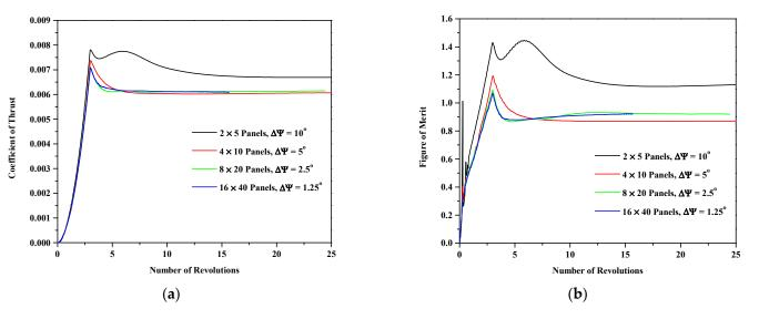
**Figure 3.** Convergence of (**a**) the coefficient of thrust and (**b**) the figure of merit for four different lifting surface and time discretizations at a collective angle of  $9.25^{\circ}$  and a tip Mach number 0.65 out of ground effect.
