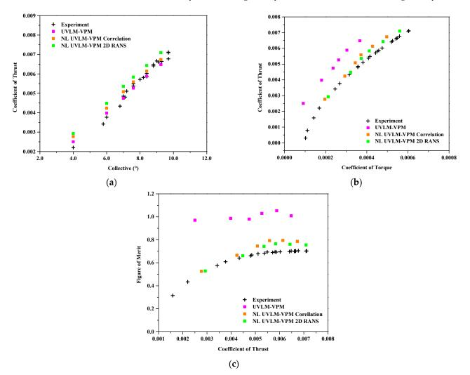
**Figure 16.** Comparisons between hybrid UVLM-VPM with experimental data. (**a**) coefficient of thrust  $C_T$  varying with collective angle, (**b**) coefficient of thrust  $C_T$  varying with coefficient of torque  $C_Q$ , and (**c**) figure of merit varying with the coefficient of thrust  $C_T$ .
