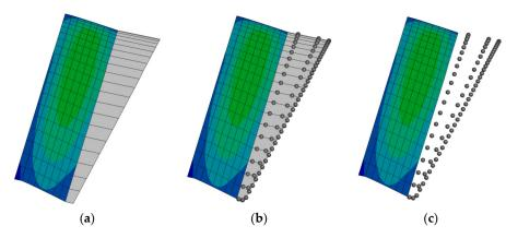
**Figure 1.** The process to convert vortex rings to vortex particles, (**a**) creation of shed wake panels, (**b**) conversion of the trailing and shed straight-line elements of wake panels to vortex particles, and (**c**) suppression of the trailing and shed straight-line elements of wake panels.
