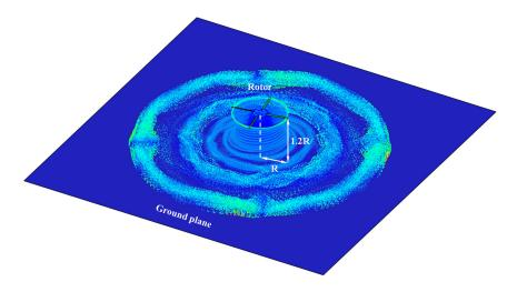
**Figure 14.** Vectorial  $\Gamma$  colored by the eddy viscosity of wake particles from the S76 rotor rotating with  $M_{tip} = 0.6$ , collective pitch angle of  $9.25^{\circ}$ , and hovering at 1.2 R from the ground plane.
