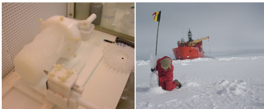
Fig. 1 Photographs of (left) ice-core cutting process and (right) sample placement for the in situ incubation. 1-cm-thick slices of sea-ice cores were cut using titanium chisels and blades under a class 100 laminar flow hood; bottom ice slices were transferred into acid-
